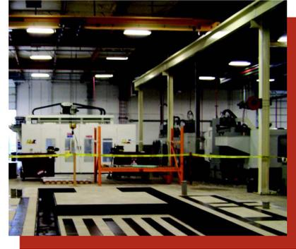
The plant, where Delta was to build the foundation for a Linx machining center, was located in an old riverbed, near potential volcanic activity. The company’s skilled engineers designed a substructure that could withstand a natural disaster and prevent any shifting of the machinery that produces precision parts with extreme tolerances as small as ten thousandths of an inch.
